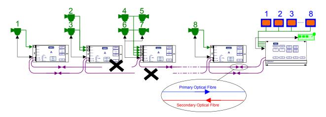
Note that where necessary repeaters can be added at nodes to increase the distance between nodes.
