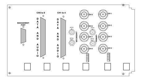
The AMG2788RN-DR-CWDM6/8 is designed to operate with AMG2783-1-DR-CWDM6/8, AMG2783-2-DR-CWDM6/8, AMG2783-4-DR-CWDM6/8 and AMG2783-DR-CWDM6/8, single channel, dual channel, 4 channel and 8 channel video and bi-directional data insert units respectively or their rackmount equivalents. Each receiver will 'drop off' up to eight video channels that are being transmitted around the single fibre ring. When used with an 8-channel transmitter the ring becomes a point to point system.
