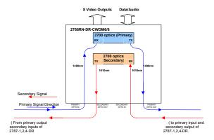
In normal operation, where connection of both the previous unit and the subsequent unit are OK, the video and data signal is taken from the primary input and the data transmitted out on the primary output. The secondary optical input is independent and is regenerated on to the secondary output.
