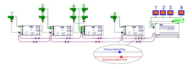
If a fibre link is broken, operation of the ring continues by making use of the secondary optical fibre route as below:
